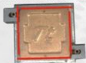
Position of the welding material
